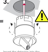
Insert the detector into the cutout. Take special care when bending the springs back
