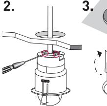
Attach the cable clamp.
