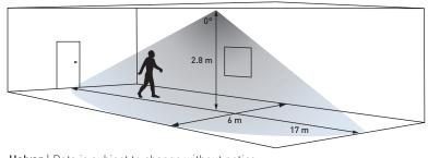
Detector head position at  $0^{\circ}$  to the vertical for open plan areas and offices. Sensitivity set to maximum.
